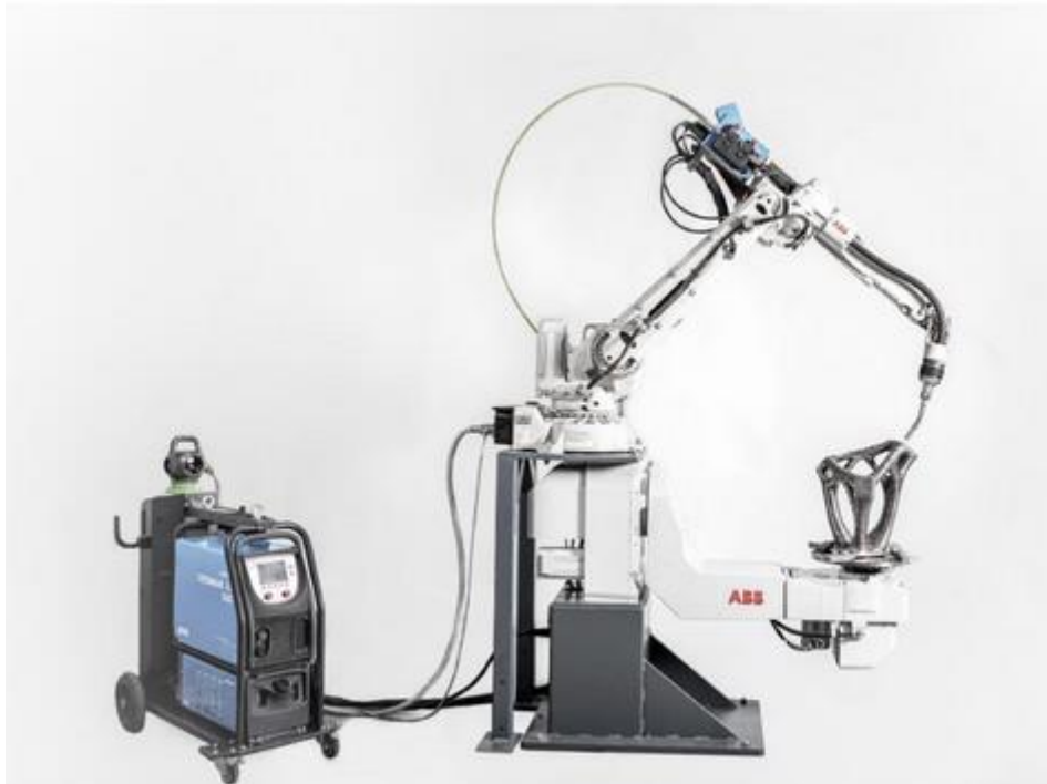
Typical Wire+Arc Additive Manufacturing setup at MX3D
