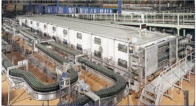
Figure 1: Tunnel pasteurizer in a beer bottle packaging line
