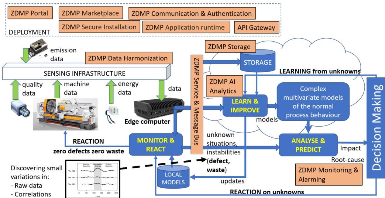
ZeroWasteZDM high-level architecture. Blue: ZeroWasteZDM custom functionality, Orange: ZDMP zComponents
